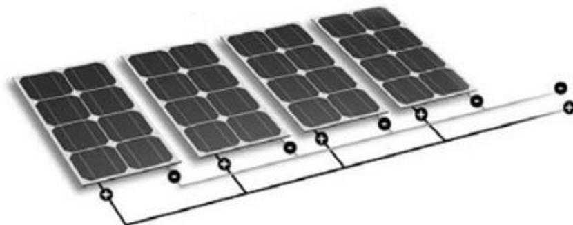
6.10 Open the connection box of the control system and connect the cabled from the PV arrays to the connection box in accordance with the installation indication of the PV control systems.
